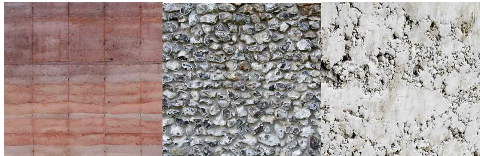
REAL 'HEAVY' MATERIALS WITH LOW EMBODIED CARBON – RAMMED EARTH – STONE – FLINT - CHALK
